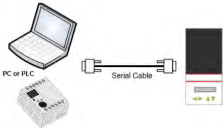
Figure 1: RS-232 Serial Interface with PC or PLC to a TriStar controller
